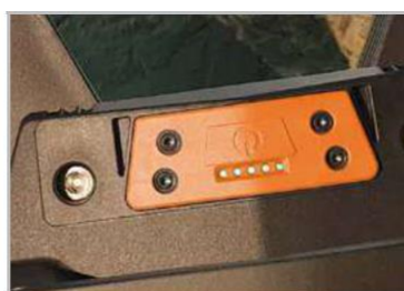
Battery Level Indication on battery pack via 5 LED battery level indicator. Each Led indicates 20% charge
