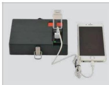
Rechargeable &amp; removable battery pack can also be used as a power bank
